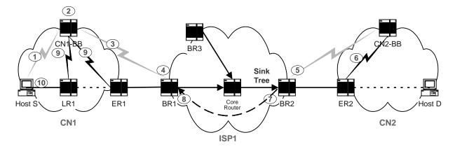
Figure 5. The signaling process of dynamic Premium Service in a MPLS-based architecture
